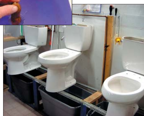
The newly encased testing media (see inset) for the MaP toilet testing protocol are reusable and leave the water clean enough to reuse too, dramatically reducing the amount of soybean paste and water needed to test each model. Photo: John Koeller, P.E.
