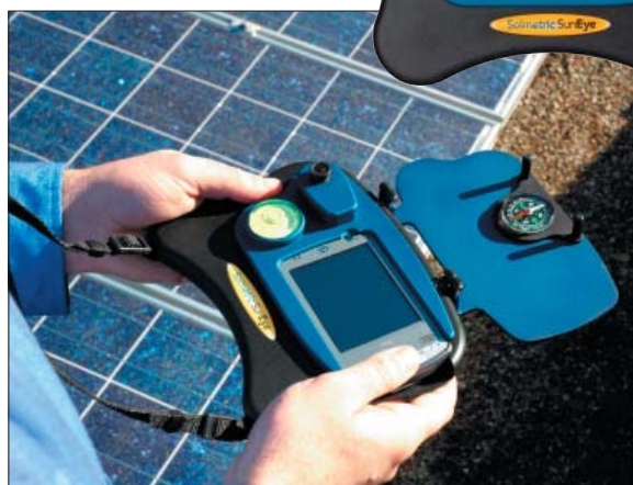
The SunEye uses digital camera technology and a sophisticated processor with computer interface to assess solar access quickly and easily.
