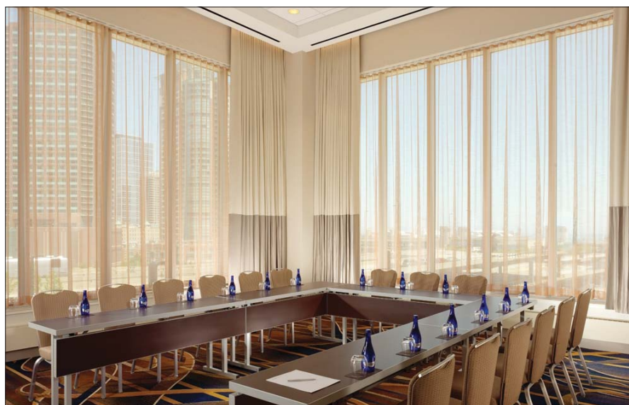
The drapes in this Swiss hotel use Trevira CS, which has non-halogenated flame retardants built into the fiber.
