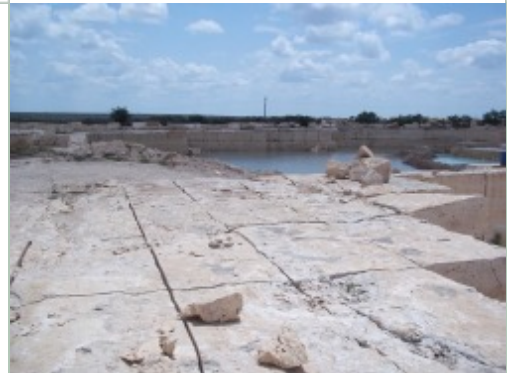
Located in the Permian Basin in Texas, site of an ancient sea, TexaStone Quarries' limestone sits on the surface; its quarrying requires almost no removal of topsoil or vegetation.
