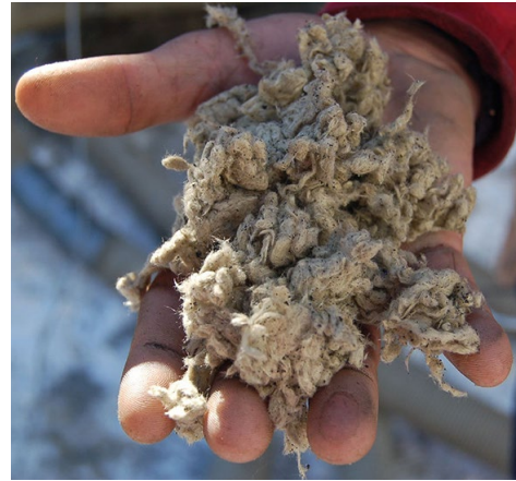
In this mineral wool sample, you can see flecks of black—bits of residual iron from the blast furnace.
