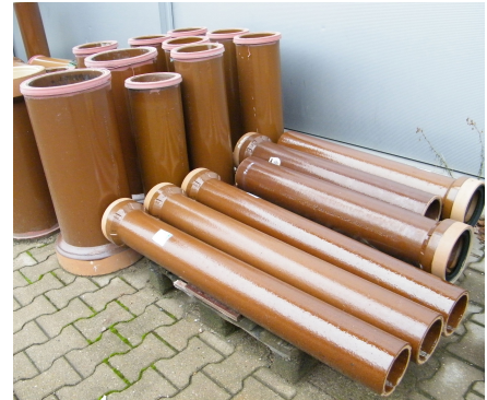
Vitrified clay is an ultra-low-impact piping solution for certain applications.
